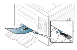
• In the software application, set the margins to at least 6.4 mm (0.25 inches) away from the edges of the material.
